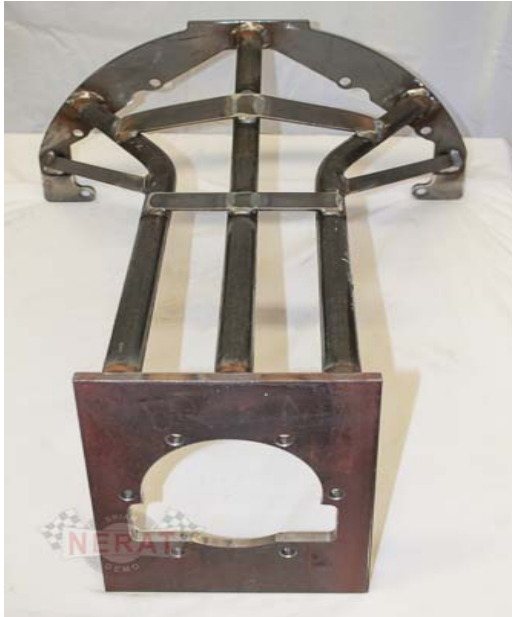
Example of trans braces allowed.
